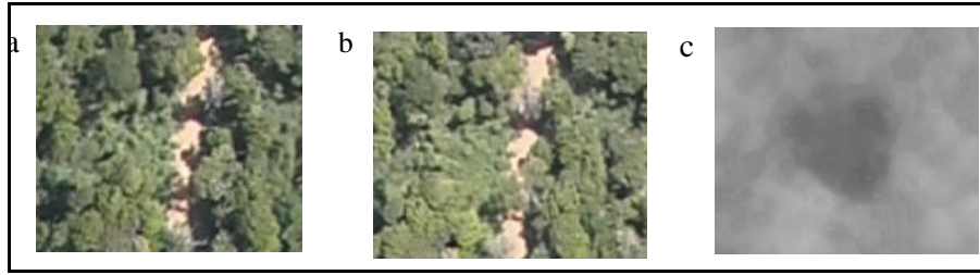
Figure 1.15. Close-up windows of the wide angle stereo mosaics in Figure 1.14 show much lower resolution of trees and largely different illuminations, perspective distortions and occlusions in (a) the left and (b) the right mosaics, and hence produce (c) less accurate 3D results.
