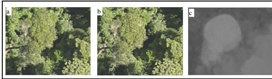
Figure 1.13. Close-up windows of the telephoto stereo mosaics in Figure 1.12 show high resolution of the trees and good appearance similarity in (a) the left and (b) the right mosaics, and hence produce (c) good 3D results.
