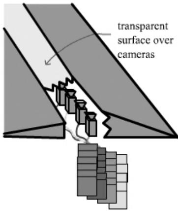
Figure 2. Camera platform of the UVIS system.
