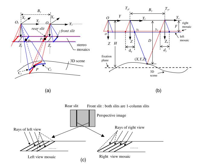
Fig. 1. The model of stereoscopic mosaics. (a). Left (blue) and right (red) views. (b). Stereo disparity geometry (side view). (c). Parallel-perspective stereo geometry: In each mosaic, each column is a full perspective projection, but successive columns have different viewpoints.
