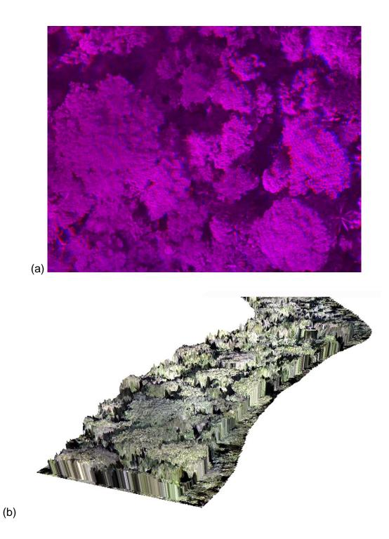
Fig. 5. Applications of stereo mosaics. (a). Stereoscopic viewing: red-blue overlaid stereo pair (Better stereo effect in the electronic version). (b). 3D rendering result: 3D recovery using stereo mosaics.
