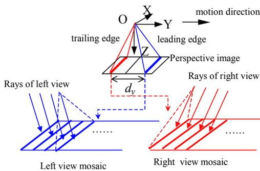
Fig. 1. Principle of the pushbroom stereo mosaics
