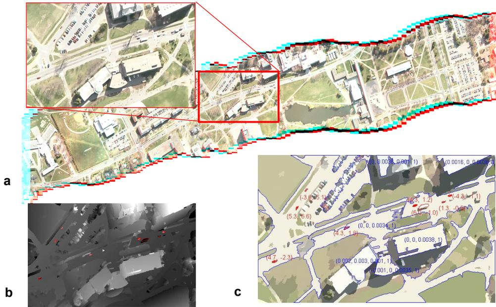
**Fig 6. Content-based 3D mosaic representation of an aerial video sequence. (a) A pair of stereo mosaics from the total nine mosaics and a close-up window; (b) the height map of the objects inside that window; (c) the CB3M representation with some of the regions labeled by their boundaries and plane parameters (in blue), and the detected moving targets marked by their boundaries and motion vectors (in red).**
