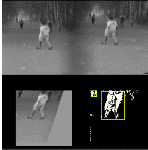
(a)Left image, right image, left reprojected image and obstacle regions in the difference image (two obstacle are detected)
