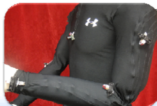
Figure 3: Recent prototype consisting of 7 sensors and vibrators connected to a central control box.
