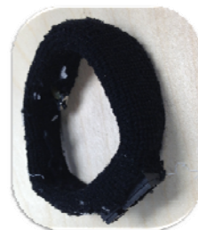
Figure 6: Analog vibrotactile pod with range sensor and vibrator
