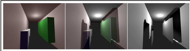
Fig. 5. Three-dimensional hand-made model of a part of a corridor at ASL representing ground truth (left). The same scene generated by the mobile robot measurement and 3D mapping algorithm (right). A superimposition of the two (center). Note that on the left side of the image a cupboard can be identified; on the right side, a group of lockers.
