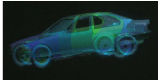
Figure 8. An image taken directly from the projection screen. It shows four images overlaid on top of each other. Two images are displayed for the left user's eyes and the other two images for the right user's eyes.
