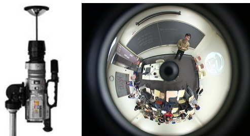
Fig. 4. The omnidirectional camera and an omnidirectional image with both the instructor and the students in view.
