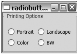
Figure 3-14. Four radio buttons in a group box. Can you tell which one groups with which?
