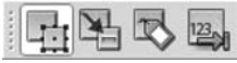
Figure 2-11. The working modes are (from left to right): edit widgets, edit connections, edit buddies, and edit tab order.
