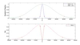
Figure 8. The Gaussian bandpass filter transfer function
