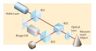
Figure 5 .The modules of the Laser Doppler Vibrometer
