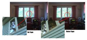
Figure 12. Listening through windows – a person was speaking outside the house, close to a window, while the LDV was listening inside the room via the window frame. Left: without retro-tape; right: with retro-tape.
