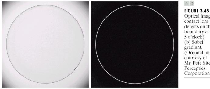
Optical image of contact lens (note defects on the boundary at 4 and 5 o'clock). (b) Sobel gradient. (Original image courtesy of Mr. Pete Sites, Perceptics Corporation.)
