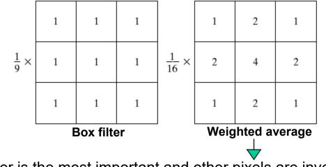
The center is the most important and other pixels are inversely weighted as a function of their distance from the center of the mask. This reduces blurring in the smoothing process.
