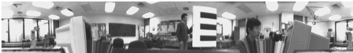
Fig. 2.4. Cylindrical panoramic image, after eliminating radial distortion
