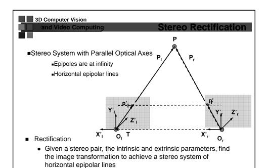
• A simple algorithm: Assuming calibrated stereo cameras
