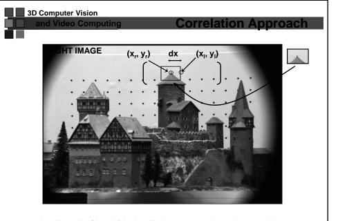
... the disparity (dx, dy) is the displacement when the correlation is maximum
