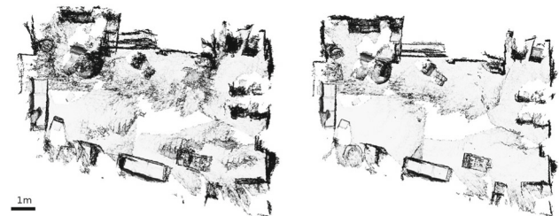
Fig. 22 Results from a 3D mapping experiment with a Google Peanut mobile device. Left: orthographic projection of the 3D map, created using data without polynomial depth calibration. Right: result from same experiment, repeated with polynomial depth image correction. Both maps are generated using pre-computed trajectories that do not rely on depth images
