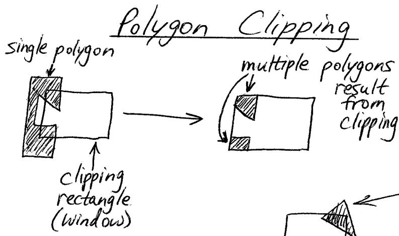
Clipping a polygon to a clip rectangle requires each polygon edge to be tested against each edge of the clip rectangle
