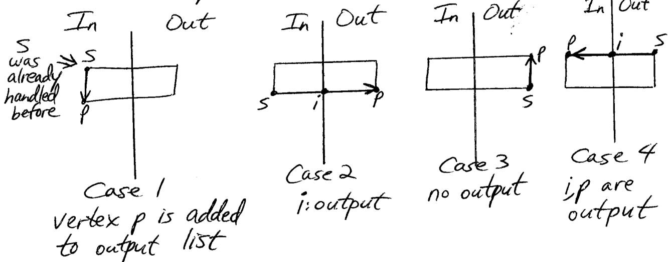
The Sutherland-Hodgman alg. is also reentrant: as soon as a vertex is output, the clipper calls itself with that vertex (to clip against next clip bdry). No intermediate storage for partially clipped polygon.
